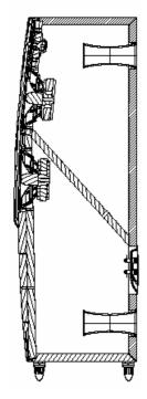
The dual bass reflex configuration means that the cabinet of D 450 is divided into two chambers – one for the tweeter/mid-woofer and one for the designated woofer. This gives several advantages: First of all the
